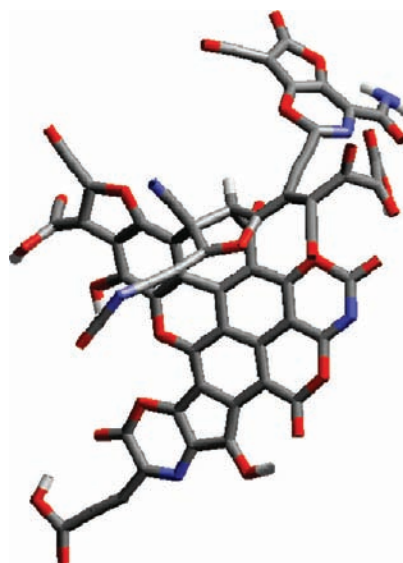
Figure 23. Final structure of the largest carbon cluster formed in 10-fold expanded TATB ( d = 0.188 \text{ g/cm}^3 ) after cooling down from T = 3000 to 500 \text{ K} . The configuration was taken from the last step of the sudden expansion simulation.
